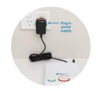
**4. Plug it in** Plug the base unit into the power point. The unit will display 'PE'. Once it's connected to the mobile network (1-2 minutes) it will announce 'Unit Disarmed' and 'PE' will clear.
